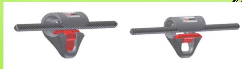
Figure 11: Glider Unlocked & Locked on the cable
